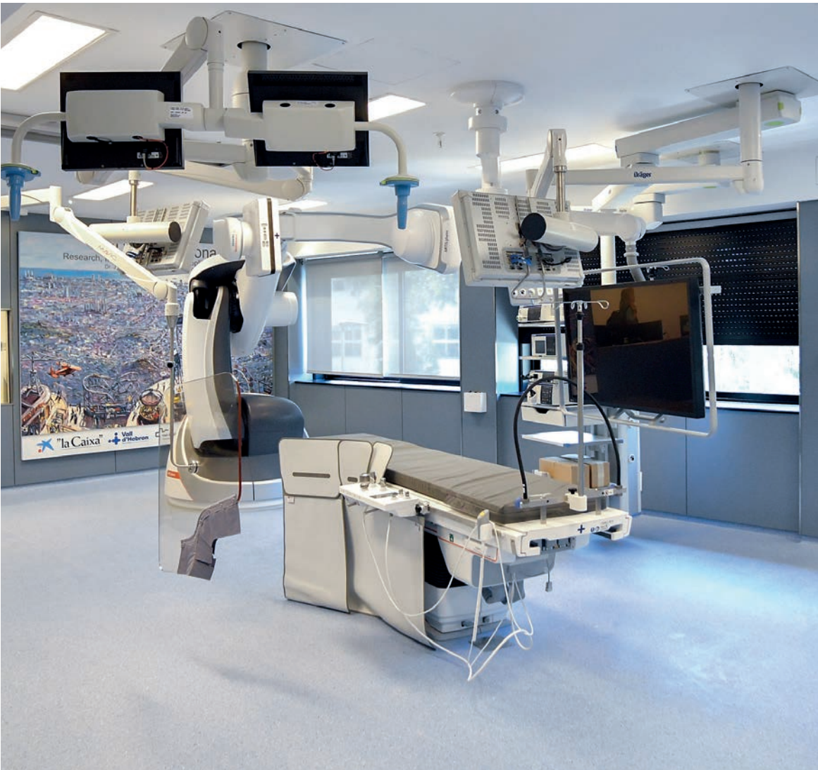
“Pheno” consists of a robotic X-ray arc, which is connected to a scanner that generates three-dimensional images that can be superimposed on those obtained by endoscopy during any chest and abdomen examination or intervention.
